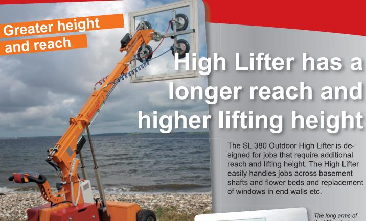
the lifting device easily reach heights where panes have be transported across e.g. fences.
