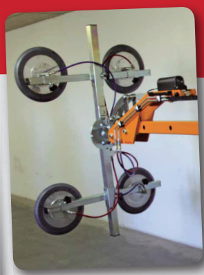
The yoke allows multidirectional movement.
