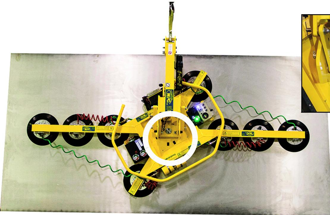
Align the secondary rotation stops for correct use of the pad frame in long, narrow configurations.
