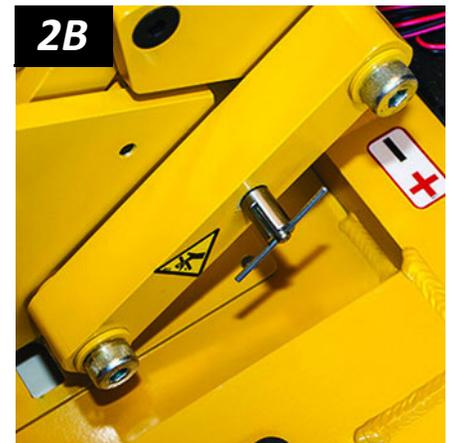
1..... These secondary safety devices do not eliminate the need to load the lifter correctly. Failure to do so could damage tilt locks or other lifter components.
