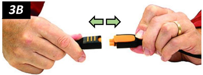
3) Disconnect the electrical connectors (figs. 3A-B and figs. 3C-E) to prevent battery discharge.
