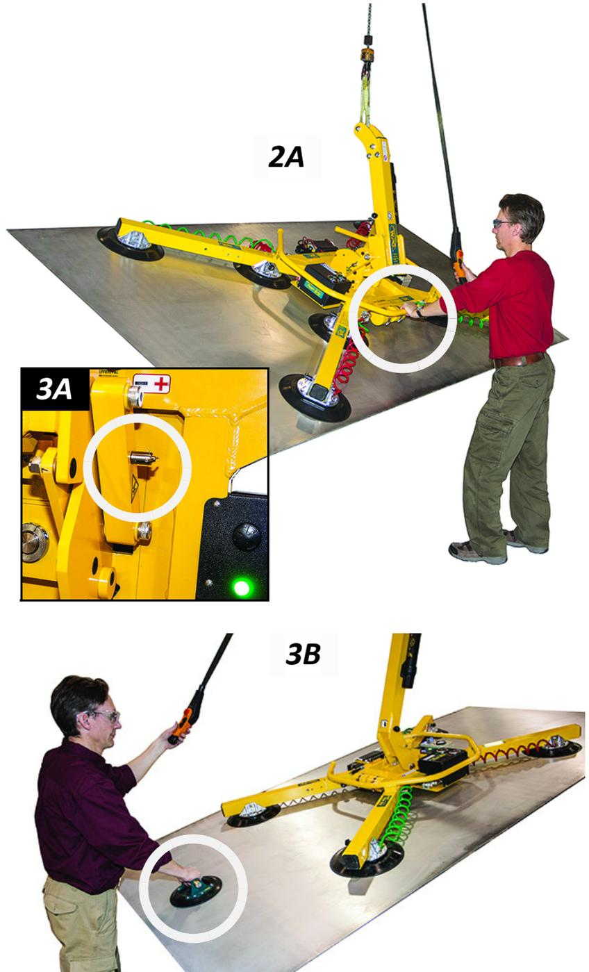
1..... Due to the tilt linkage design, load force on the control handle changes direction during the tilt.
