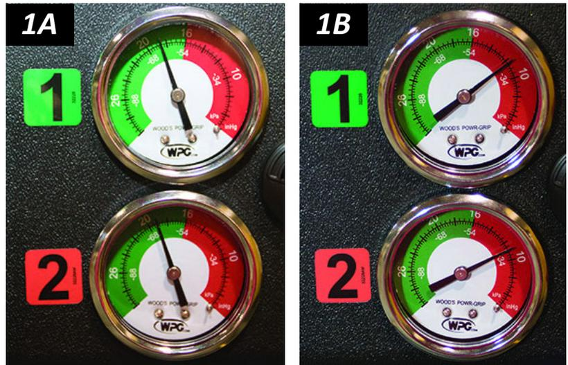
If it takes more than 5 seconds for the vacuum level to reach 5" Hg [-17 kPa] on either vacuum gauge, press on any vacuum pad that has not yet sealed.
