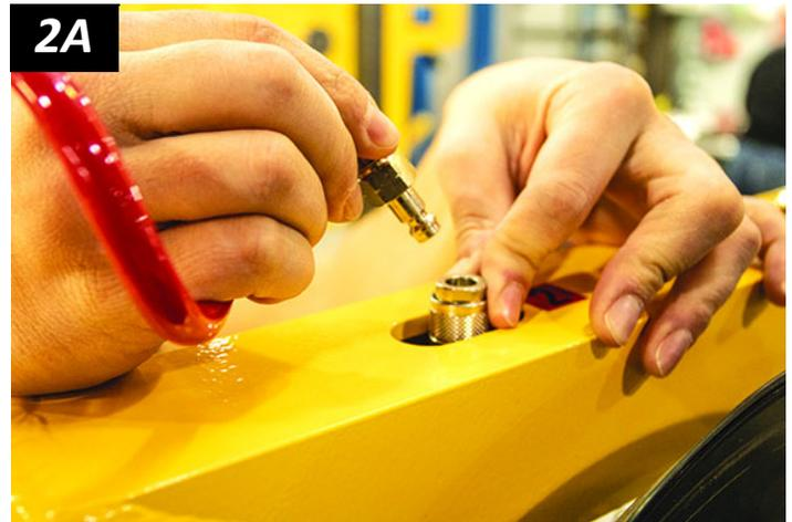
To *connect* a vacuum hose, push the male and female ends of the quick connector together until they lock (fig. 1A).
