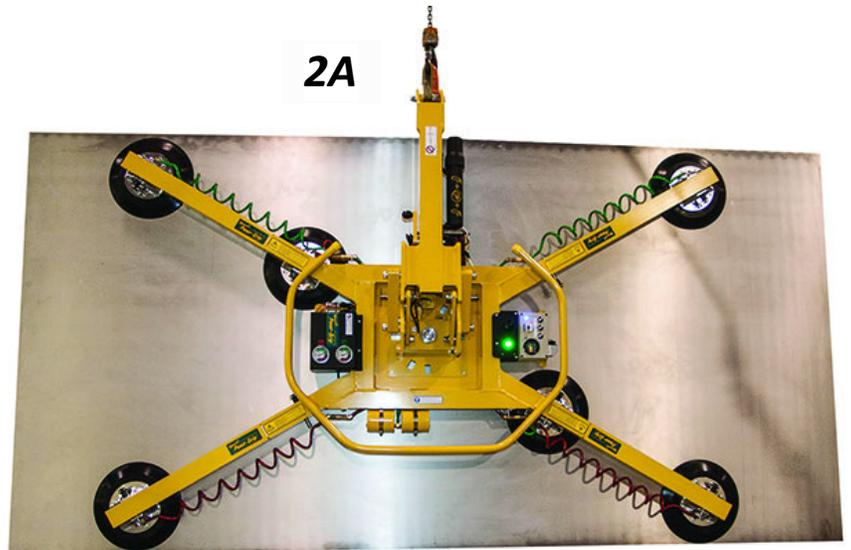
1..... The lifter is designed to handle the maximum load weight when the load's center of gravity is positioned within 2" [5 cm] of the lifter's rotation axis. Uncentered loads may rotate or tilt unexpectedly (as applicable).
