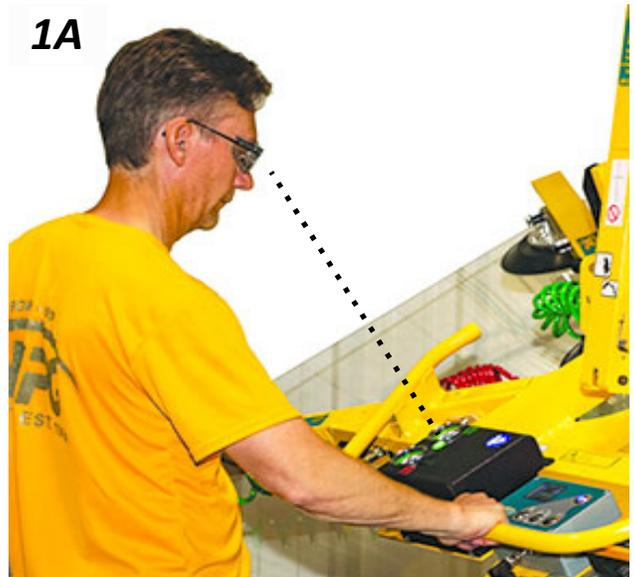
1.... Automatic leak detection is **not** a substitute for performing the “[Vacuum Test](#)”, required by the “[INSPECTION SCHEDULE](#)” and “[TESTING](#)”. Sensitivity of leak detection can be adjusted (see “[INTELLI-GRIP® OPERATOR MENUS](#)” in [SERVICE MANUAL](#)).
