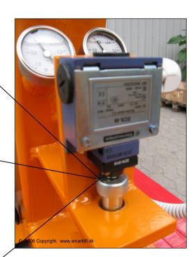
If —no response when pushing control panel, <u>individual functions</u>, Has the safety switch been activated? If activated, try one of the possibilities above. There may be a fault on actuators for movements, or when controlling these.
