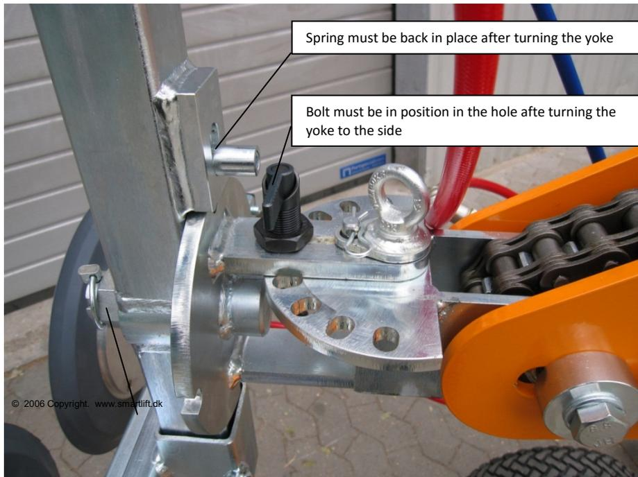
If the yoke has been dismantled, be aware that the washer is placed between the castle nut and the yoke.
