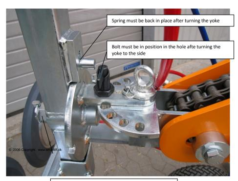
If the yoke has been dismantled, be aware that the washer is placed between the castle nut and the yoke.
