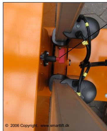
In particular lines at the bottom of these two lift actuators may, by carelessly wrong and unfortunate operation of SL-380, have been damaged at connector or line.
