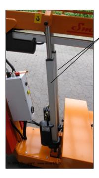
Actuators for lifting, 2 pcs. Linak LA36
