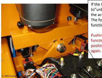
If the lift actuators, or one of these, stop due to"unbalanced" load, one of the safety switches under the actuators will have switched off the power supply. The following may be done to re-establish normal function:
