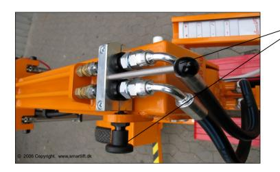
Slide Valve w/safety lock for activation and deactivation of vacuum suction.
